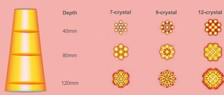
Our 12-crystal ultrasound probe employs advanced technology unique to EDAN, providing wider beam area and more homogeneous signal, thus realizing better performance for bedside monitors than conventional transducers.
